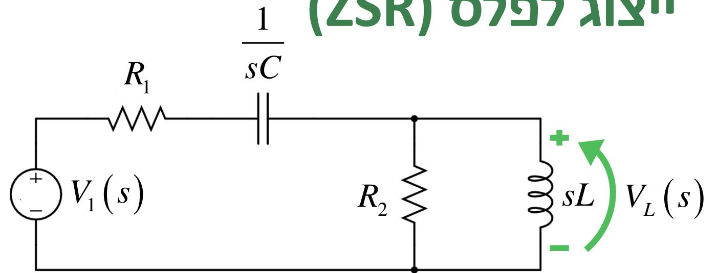
$$V_L(s) = \frac{R_2 \parallel sL}{R_1 + \frac{1}{sC} + (R_2 \parallel sL)} V_1(s)$$
