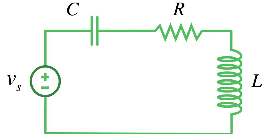
$$v_C(0) = v_0^C \quad i_L(0) = i_0^L$$
