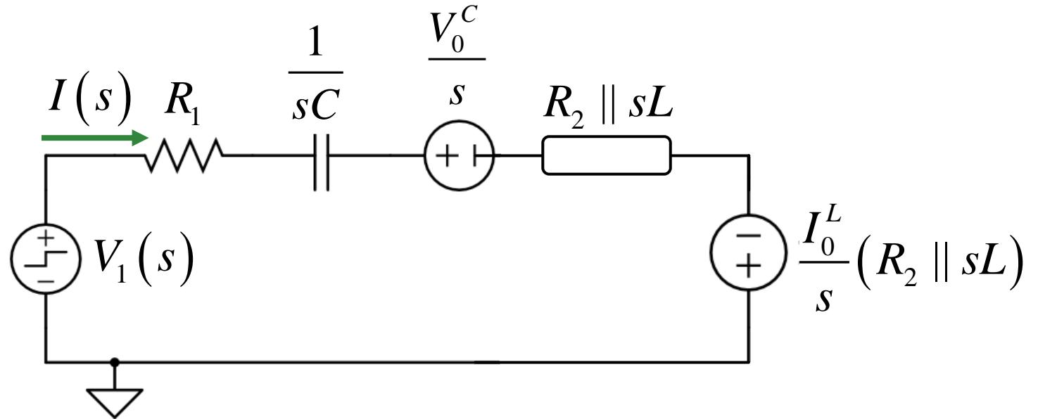
$$\left( R_1 + \frac{1}{sC} + R_2 \parallel sL \right) I(s) + \frac{V_0^C}{s} - \frac{I_0^L}{s} (R_2 \parallel sL) = V_1(s)$$
